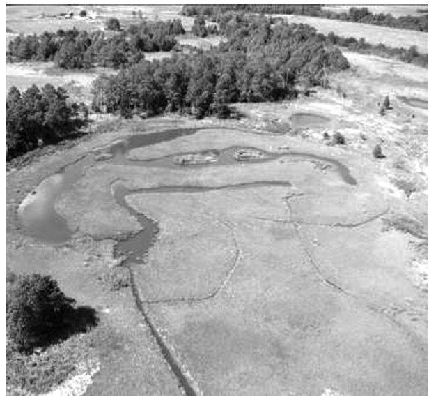
Figure 17 The OMWM system, involving the selective installation of small, shallow ponds and interconnecting ditches superimposed on known mosquito-breeding habitats.
