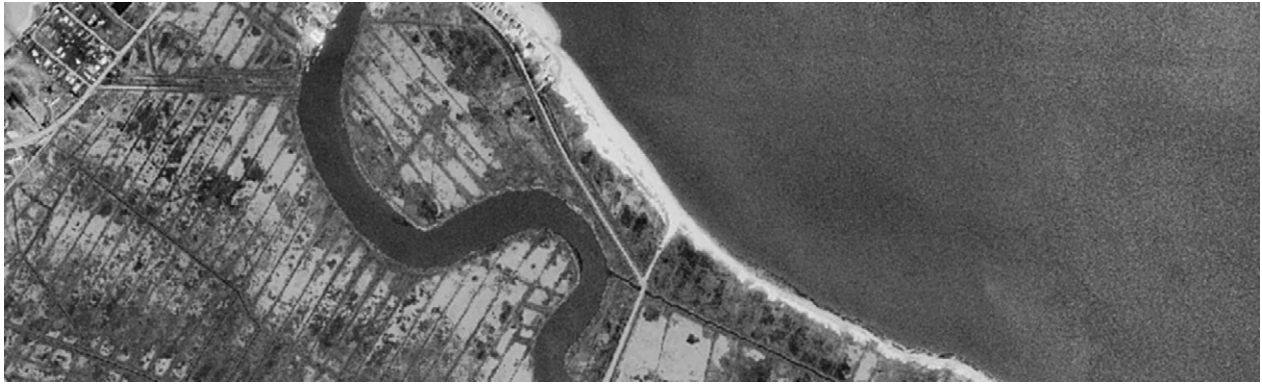
Figure 16 Network of parallel grid ditches located near Bowers Beach, Delaware. Photo taken in 1997; ditches were last cleaned in mid-1960s and remain functionally tidal today. Reproduced from Lesser, C.R., 2007. Open marsh water management: a source reduction technique for mosquito control. Delaware Mosquito Control Section.
