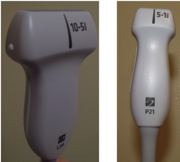
Figure 1. A high frequency linear transducer is shown on the left and a phased array probe is shown on the right.
