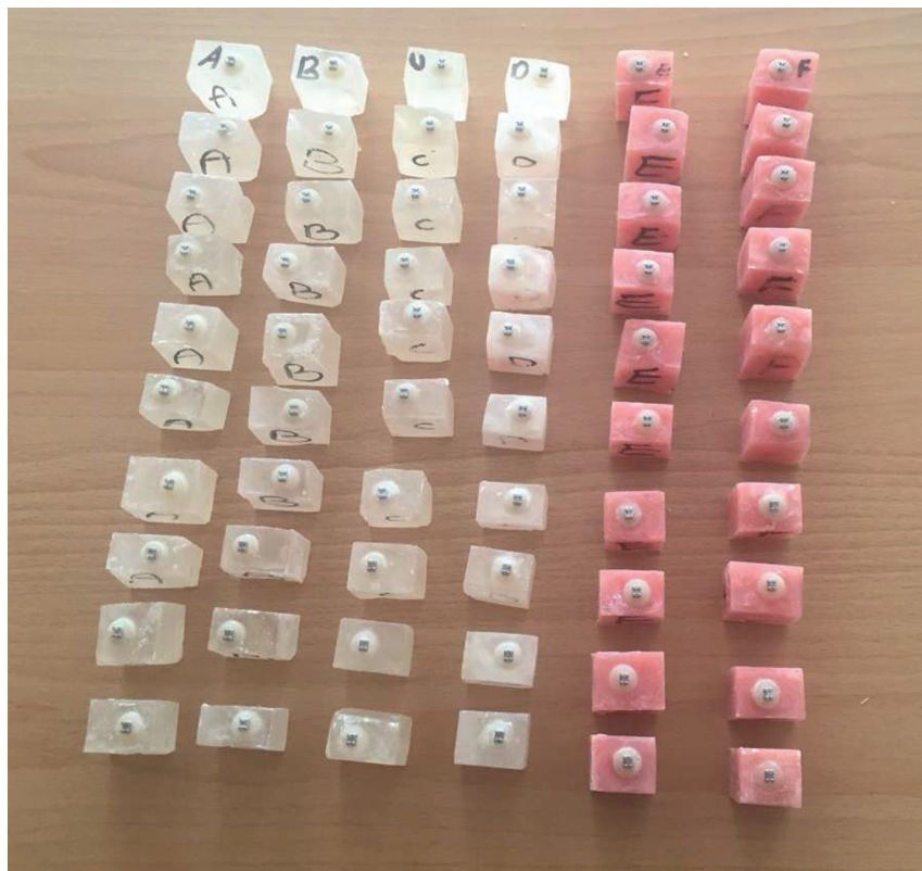
Fig. 1: Mounted samples for bond strength testing.
