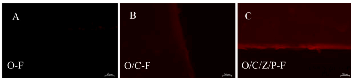
Fig. 2. Fluorescence properties of modified starch film. (A) OSCS Film (O-F); (B) OSCS/CS Film (O/C-F); (C) OSCS/CS/ZnO/ε-PL Film (O/C/Z/P-F).
