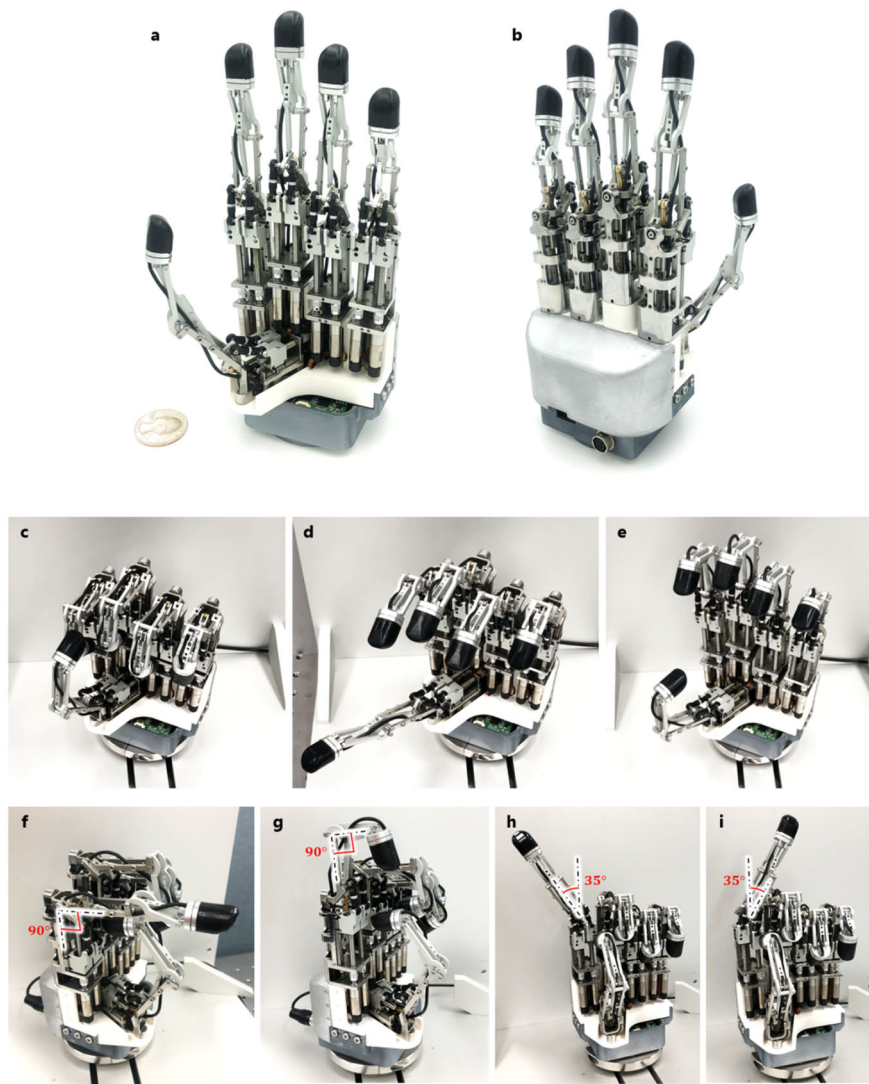
Fig. 5 Manufactured ILDA hand. a Front view. b Rear view. c–i Motion tests of the developed ILDA hand. c Fist of the hand. d, e Motions of the five fingers of the hand. f–i Maximum 3-DOF motions of the finger.
