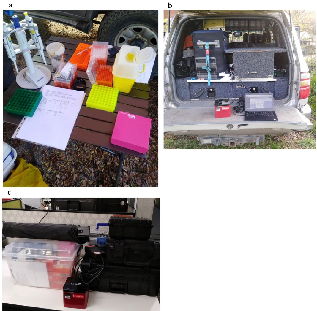
Figure 2. Deployed and functional portable laboratory set up. (a) Mid-RNA extraction in-field using the Biomeme M1 RNA extraction kit. (b) The MIC PCR machine performing that TaqMan assay out the back of the Landcruiser. (c) The entire kit packed up (all equipment listed in Supplementary data 1).
