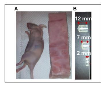
**Figure 2.** A, Slab of optical tissue equivalent phantom of mouse model consisting of slices of ham of thickness (1.5-1.8 mm). B, Radiotracer sources of <sup>89</sup>Zr in Liposyn II absorbing media placed in three different cylindrical containers with an effective depth size of 12, 7, and 2 mm inside the phantom, respectively.
