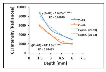
**Figure 3.** Exponential fit curve of Cerenkov luminescence imaging signal for  $^{89}$ Zr and  $^{64}$ Cu isotopes detected as a function of tissue depth used to estimate the average effective tissue attenuation coefficient.
