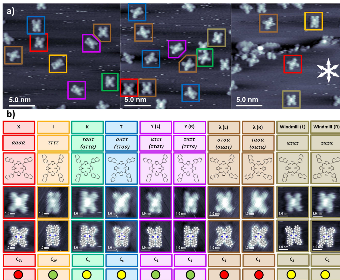
Figure 2. a) Three constant-current STM images showing the 10 surface conformations of 2HTNP highlighted by differently colored boxes. b) Name, \alpha/\tau -notation, chemical structure, high resolution STM image of a single molecule, STM image overlaid by a scaled space-filling model, point group, and mobility ranking (red: immobile, yellow: medium, green: fast) for all possible conformations. In case of equivalent rotamers, two \alpha/\tau -notations are denoted.
