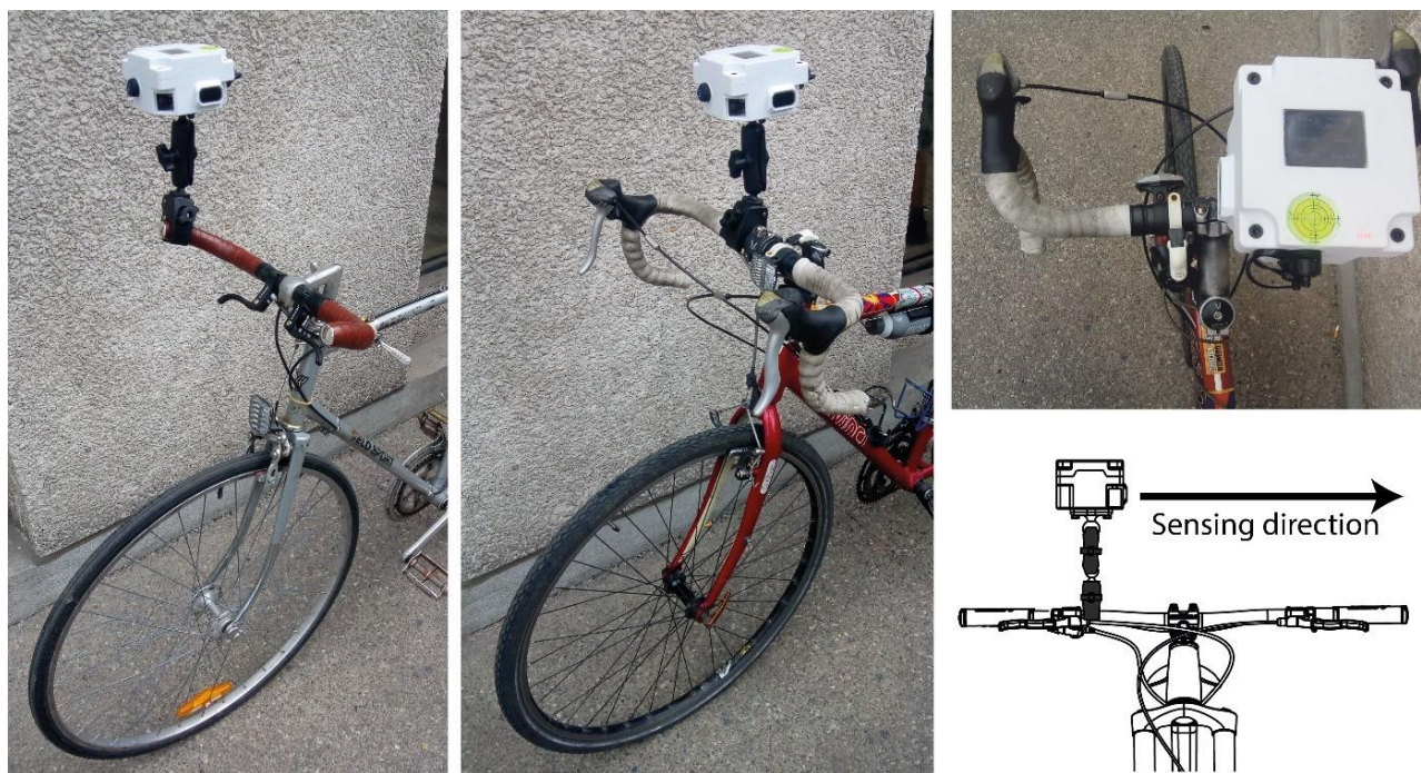
Figure 3. Integration of the one metre plus sensor to the bicycles.
