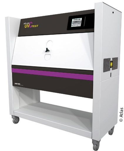
With irradiation centered on 254 nm wavelength, the influence of disinfection measures can be simulated by UV-C radiation.
