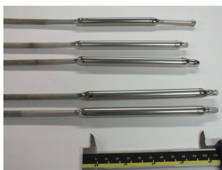
Figure 5. The \leq 1 \mu\text{m} -thick Pd-Ag-supported membranes onto \text{ZrO}_2 3-nm tubular supports.
