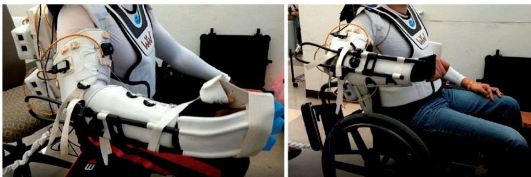
Figure 5. Test Subjects T1 (left) and T2 (right) perform rehabilitation exercises to demonstrate Armstrong's capabilities. T1 was seated on a flat bench in an upright position; T2 remained in his personal wheelchair with arm supports removed.
