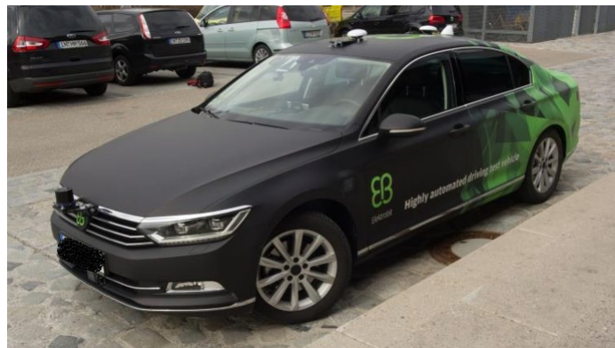
Figure 12. Test vehicle used for data acquisition and testing for the Most Probable Path (MPP) AI Inference Engine.
