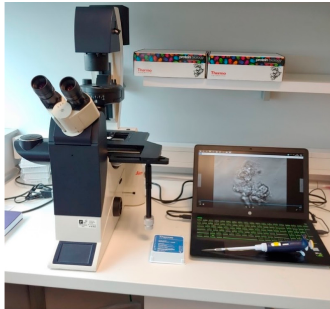
Figure 3. Leica DMI3000B inverted microscope (Berlin Germany) with system for recording and analyzing ciliary motility.
