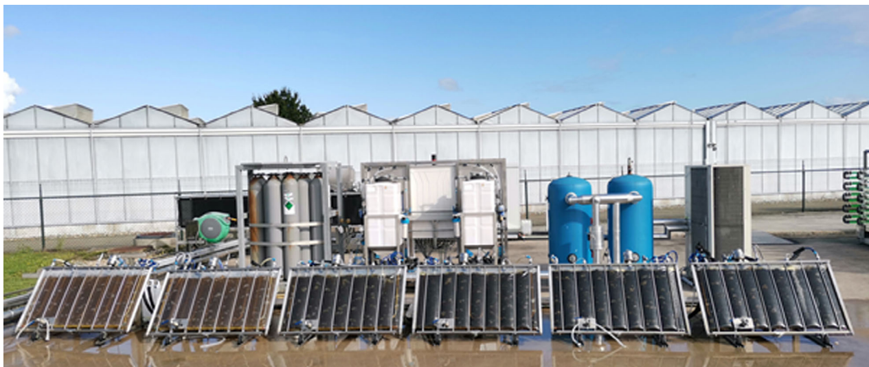
Fig. 4. Tisochrysis lutea : different biomass concentrations, from more diluted (left) to more concentrated (right), in pilot-scale outdoor production at AlgaePARC (Green Wall Panel® III, F&M Fotosintetica & Microbiologica S.r.l., Italy).
