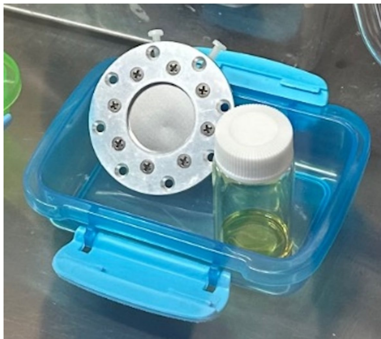
Fig. 2. A solution sample of 1 in degassed THF (0.060 M) sealed in a \mu SR sample cell.
