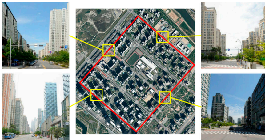
Figure 7. Driving environment in an urban environment with multipath effect that interferes with GNSS satellite signals due to high buildings.
