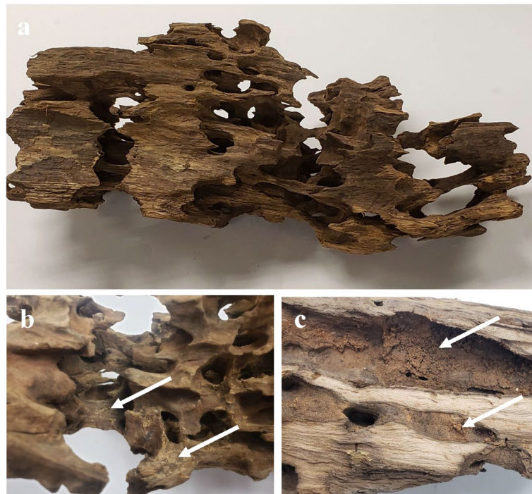
Fig. 2. Samples sold as driftwood were pieces of tropical woods that had substantial degradation resulting in holes throughout the wood. The holes make the wood attractive for use in aquariums (a). The inner zones of this decayed wood often had residual mud and soil present (b and c).
