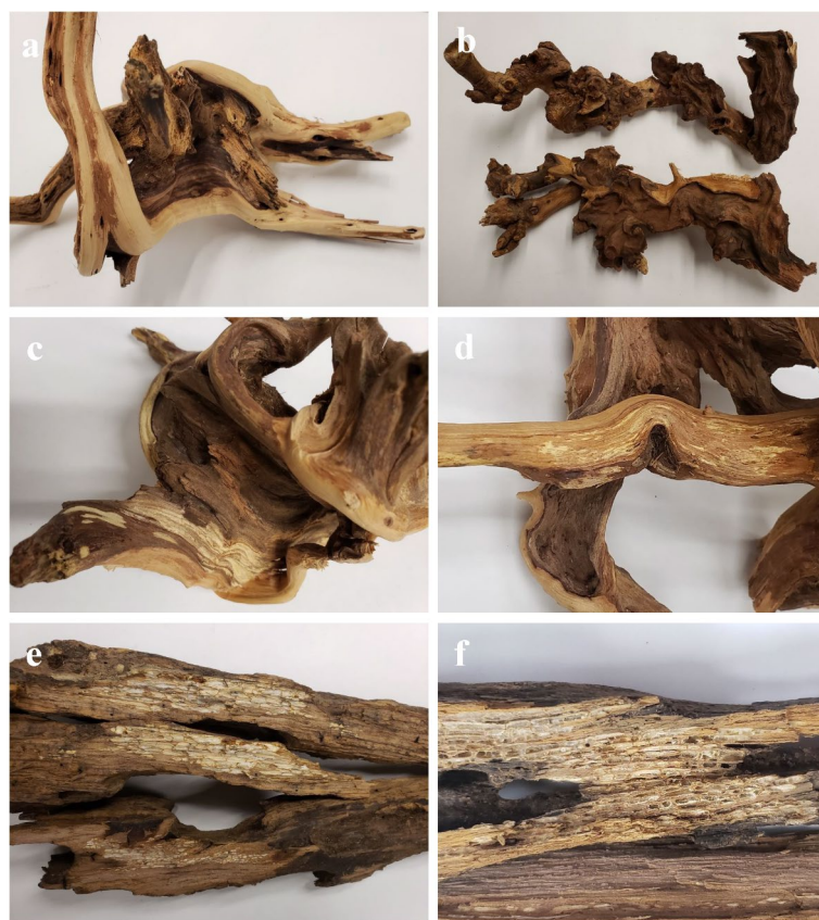
Fig. 1. Wood samples sold for aquarium decorative purposes and used for culturing fungi showing evidence of fungal colonization and decay. Dark colored areas of dead wood were present along with lighter colored sapwood (a and b). The older dead wood was the location where many fungi were isolated. White rot was present in many samples (c–f) and fungi produced incipient decay leaving a bleached white appearance (c and d) or zones of advanced decay (e and f). A white pocket rot was evident inside several of the samples that were split open for isolation and culturing (e and f).
