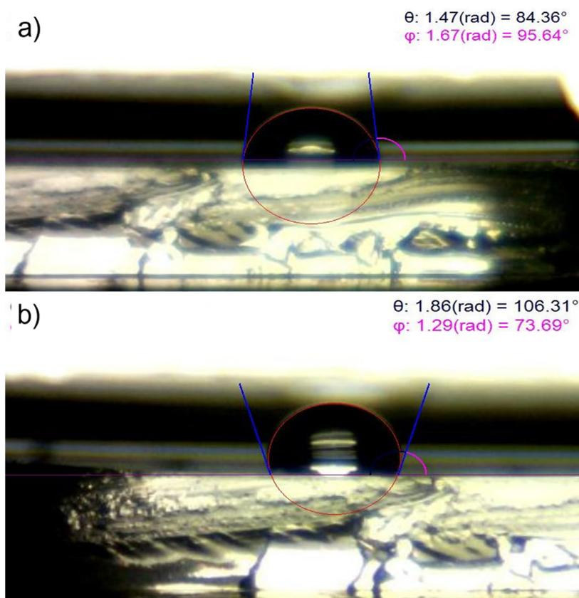
**Figure 4.** Contact angle measurement of the untreated and UV/O treated PDMS. UV/O treatment of the PDMS surface decreased the contact angle to  $84.36^\circ$  and makes it more hydrophilic (a) compared to the Untreated PDMS surface which is hydrophobic with contact angle about  $106.31^\circ$  (b).
