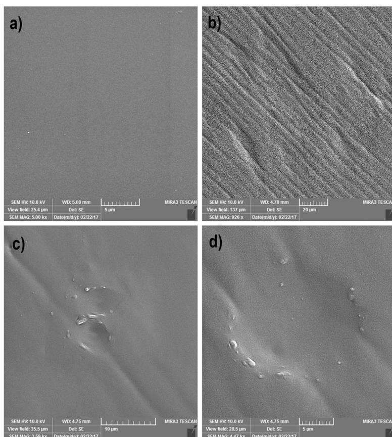
**Figure 3.** SEM image analysis of the negatively keratinocyte cell-imprinted PDMS substrate. (a) is the representative for the plane control PDMS substrate without imprinted groove. (b-d) Shows the formation of the successful grooves similar to the keratinocyte cell shape and morphology with an about 17.05 µm diameter.
