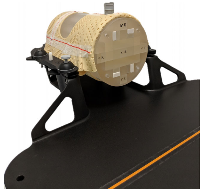
FIG. 3. MTSI SRS E2E phantom placed inside the QFix Encompass SRS headboard and mask system.
