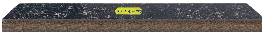
Figure 2. Sandwich composite sandwich test specimen with a 60% Dammar hybrid resin matrix, which has a shredded sunflower seed core and flax fabric surfaces, which was tested for bending in 3 points.
