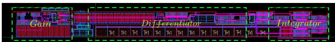
Figure 25. The layout of the integrator-differentiator transimpedance amplifier (TIA) in 130-nm CMOS.
