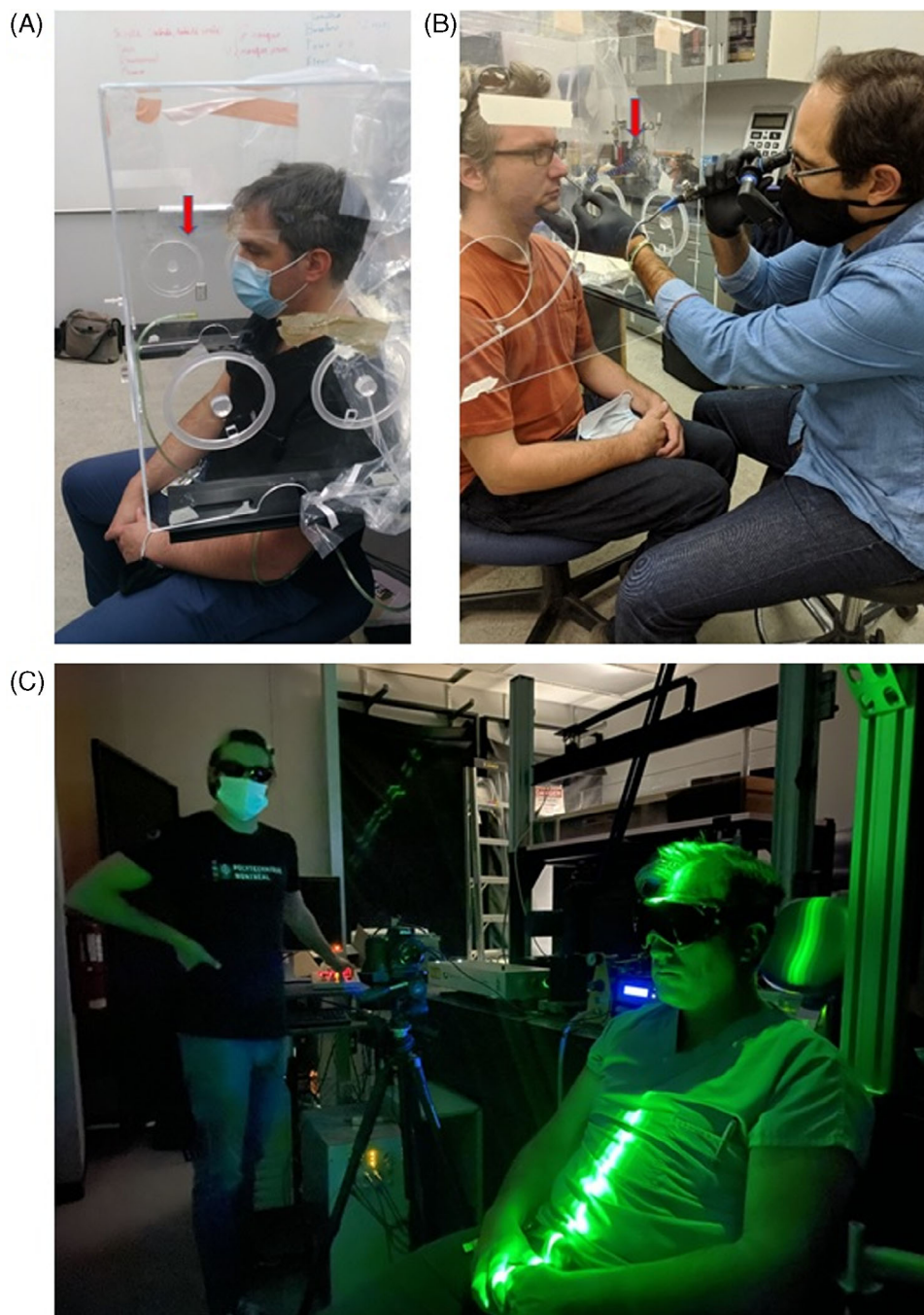
FIGURE 1 Experimental setup. The experimental setup for laser aerosol spectrometry viewed from the right (A) with the laser aerosol spectrometer (LAS) aspiration tube (red arrow) fixed 10 cm in front of the participant. The experimental setup for laser aerosol spectrometry viewed from the front left side with the circular doors (red arrow) opened for the practitioner to perform a flexible laryngoscopy without interfering with aerosol measurements (B). The experimental setup for live aerosol imaging showing the positioning of the camera, green laser sheet and participant (C).
