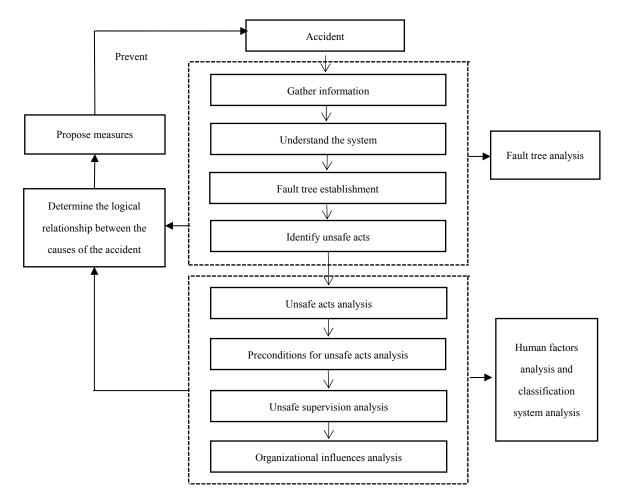
**Figure 1.** Combination of fault tree analysis (FTA) and the Human Factors Analysis and Classification System (HFACS).
