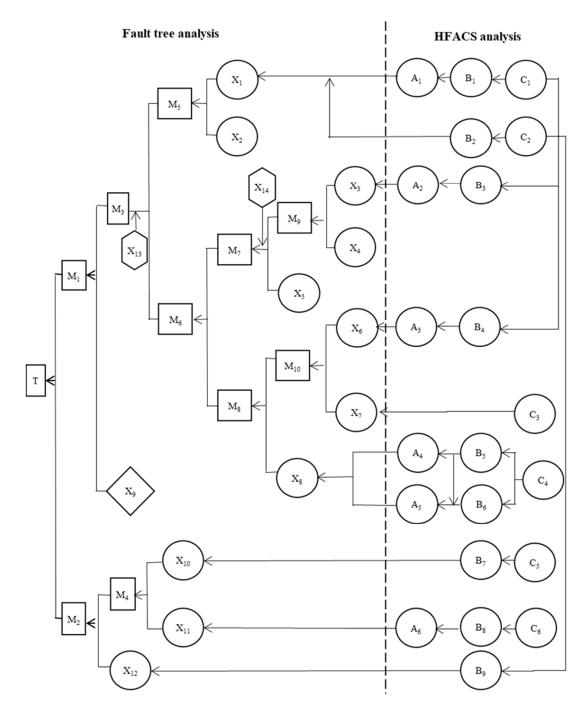
Figure 3. Logical diagram of accident causes.
