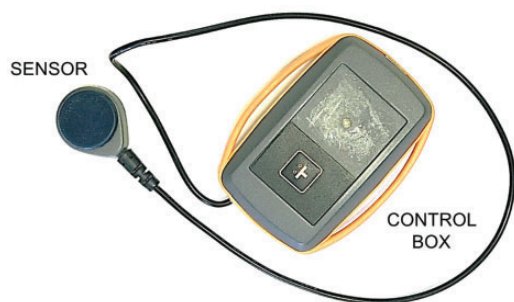
Figure 1. Prototype NIVA device consisting of a piezoelectric sensor and control box.
