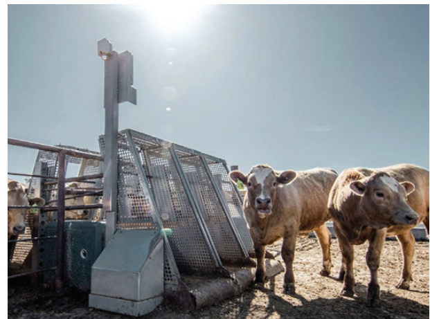
Figure 1. Operational system for the capture of partial body weight data from growing beef animals.
