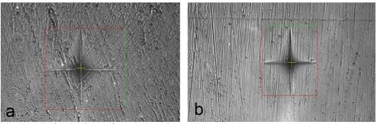
Figure 3. Surface hardness of group (A) and group (B).
