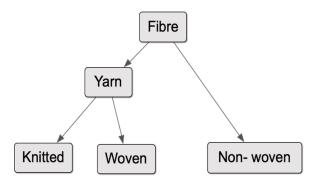
**Figure 11.** Structural map of basic textiles based on scale—fibres are the basic building block that can be applied to all fabric structures; i.e., knitted and woven textiles via yarns and directly into non-wovens.
