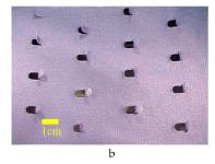
**Figure 5.** Photograph of original pinecone effect textile in dry (**a**) and damp (**b**) conditions. Sample size is  $10 \times 5$  cm. Pores open when the hygroscopic polyether layer swells on exposure to moisture vapour.
