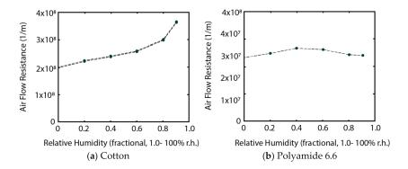
**Figure 10.** Results from cotton and nylon samples tested using by Phil Gibson, US Army Natick Soldier Systems, Natick. (a). 100% Cotton. Weight: 150 g/m², source: Paolo Gilli, cira: Spring/Summer 2004 reference: Sirena, Width: 148–150 cm (b). 100% Polyamide 6.6 Weight: 83g/m², source: William Reed, circa: 2001, reference: 131980, width: 155 cm.
