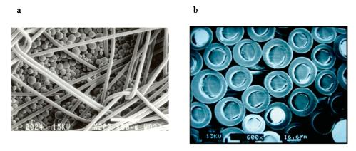
**Figure 2.** Phase change microcapsule applied onto textile as a coating (a), magnification 200×. Phase change material incorporated into the core of a fibre (b), magnification 600×. Source: Outlast Technologies.
