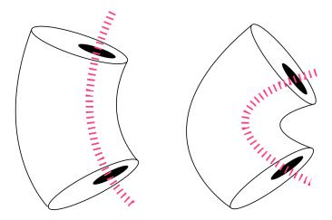
**Figure 14.** Visualisation of active fibre behaviour in dry (**left**) and damp (**right**) conditions. The antagonistic forces created between the Nylon 6 (N6), which elongates in damp conditions and the stiff, hydrophobic polypropylene (PP) cause the fibre to bend, defined as an increase in angel of crimp in the textile industry.
