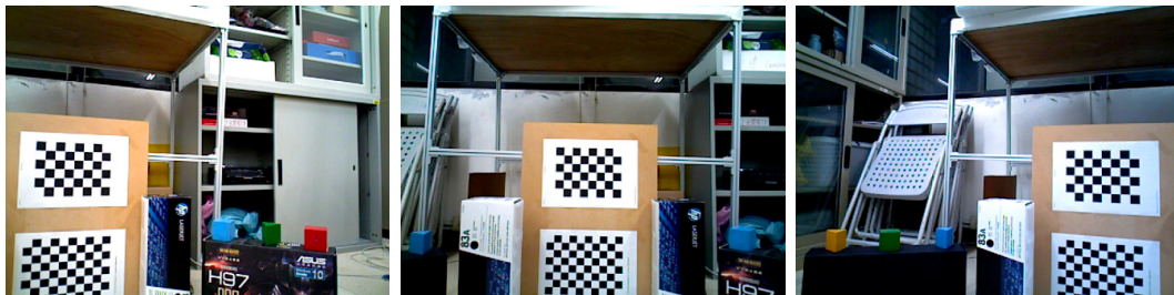
Figure 6. Illustration of the scene of point alignment calibration that is used in offline calibration. These scenes contain the same geometric objects.
