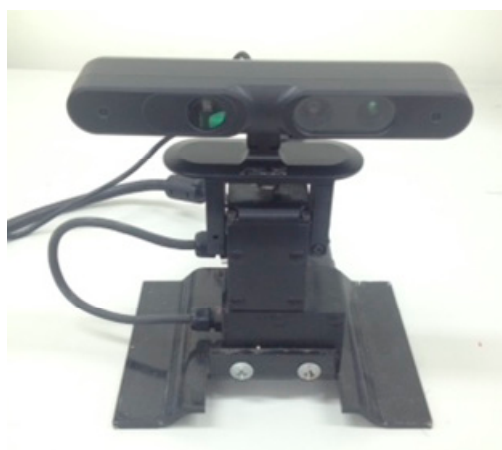
Figure 7. The physical pan-tilt device used in the experiments, which is an ASUS Xtion Pro RGB-D camera [39] mounted on an E46-17 pan-tilt platform [40].
