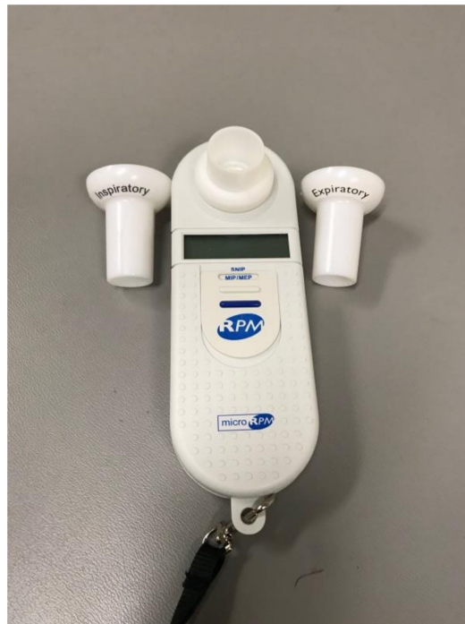
Figure 2. Maximal inspiratory pressure (MIP) and maximal expiratory pressure (MEP) device.
