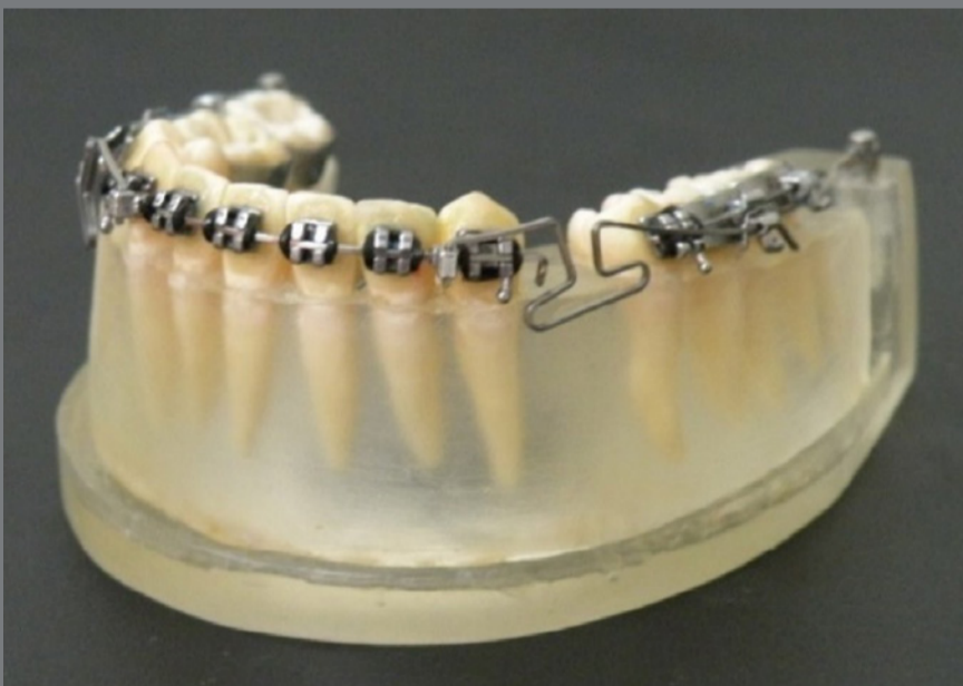
Figure 3: "T" loop spring test specimen.
