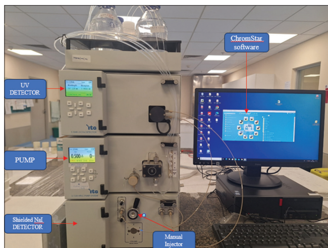
Figure 2: High-performance liquid chromatography system with its components and software
