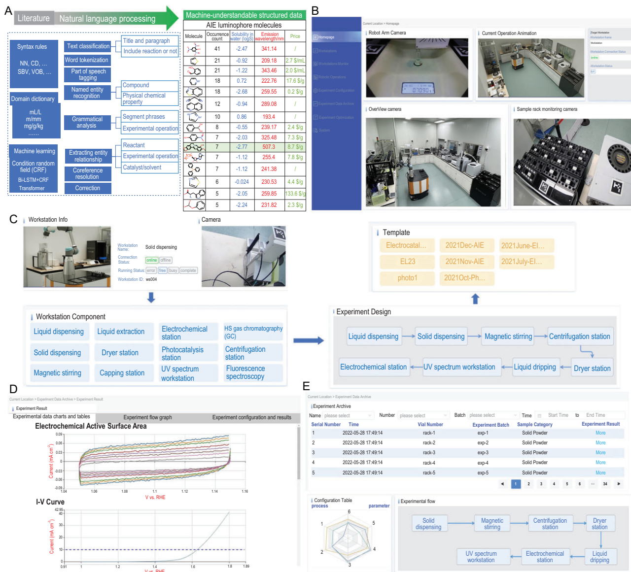
Figure 2. The service platform with web browser-based HMI. (A) Machine-reading module for capturing existing knowledge and transferring to machine-understandable structured data by NLP. (B) User-friendly GUI to monitor the status of chemical workstations and robots in real time. (C) Experimental workflow diagram: from scientific hypotheses to workstation status, then to experimental design and template. (D) Experimental data such as electrochemical active surface area and current–voltage curve collected and displayed on the service platform. (E) Experimental archives for building the experimental database and training the prediction model.
