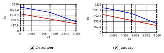
**Figure 19.** Condensation and evaporation amount chart for the building elements of the brick external wall for the 2nd zone for (a) December and (b) January.
