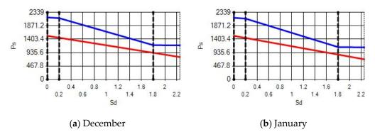
**Figure 14.** Condensation and evaporation amount chart for the building elements of the AAC external wall for the 1st zone for (a) December and (b) January.
