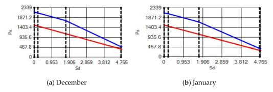
**Figure 21.** Condensation and evaporation amount chart in the building element of the brick external wall for the 4th zone for (a) December and (b) January.
