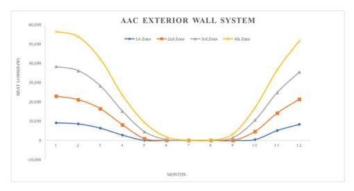
Figure 8. Heat losses for AAC exterior wall system.
