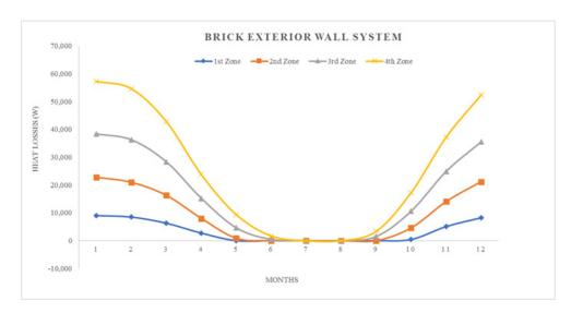
$\textbf{Figure 10.} \ \ \text{Heat losses for brick exterior wall system}.$
