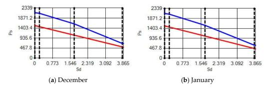
**Figure 24.** Condensation and evaporation amount chart for the building elements of the pumice external wall for the 3rd zone for (a) December and (b) January.
