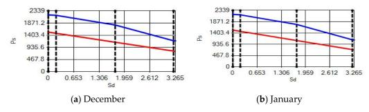
**Figure 15.** Condensation and evaporation amount chart for the building elements of the AAC external wall for the 2nd zone for (a) December and (b) January.
