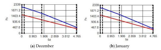
**Figure 25.** Condensation and evaporation amount chart in the building elements of the pumice external wall for the 4th zone for (a) December and (b) January.
