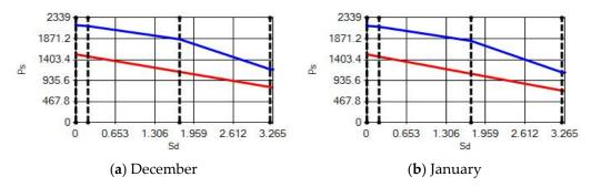
**Figure 18.** Condensation and evaporation amount chart in the building elements of the brick external wall for the 1st zone for (a) December and (b) January.
