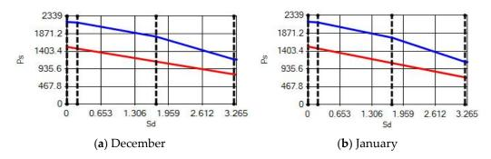
**Figure 22.** Condensation and evaporation amount chart for the building elements of the pumice external wall for the 1st zone for (a) December and (b) January.
