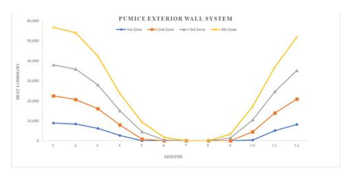
Figure 12. Heat losses for pumice exterior wall system.
