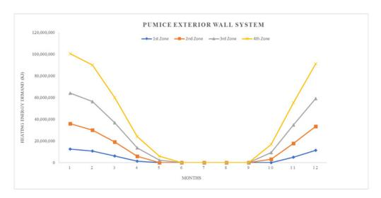
Figure 13. Heating energy demand for pumice exterior wall system.
