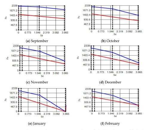
**Figure 20.** Condensation and evaporation amount chart in the building elements of the brick external wall for the 3rd zone for (a) September, (b) October, (c) November, (d) December, (e) January and (f) February.
