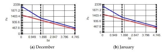
**Figure 17.** Condensation and evaporation amount chart for the building elements of the AAC external wall for the 4th zone for (a) December and (b) January.
