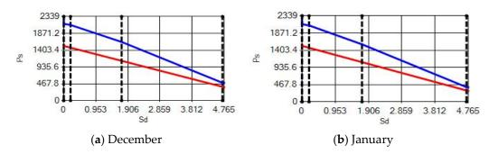
**Figure 23.** Condensation and evaporation amount chart for the building elements of the pumice external wall for the 2nd zone for (a) December and (b) January.
