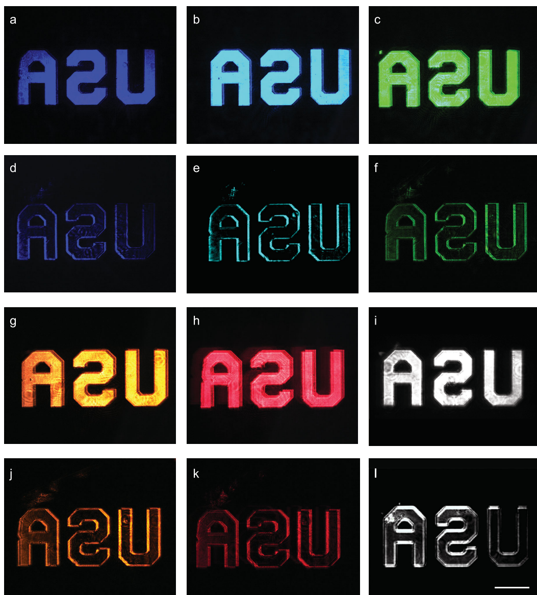
Figure 4. 2D edge detection demonstration of intensity object (R3L3S1N Negative 1951 USAF Target). (a–c and g–i) The result is taken by removing the second polarizer. (d–f and j–l) Edge images at wavelengths of 410 nm, 490 nm, 540 nm, 590 nm, 690 nm and white light, respectively. Scale bar: 1 mm.
