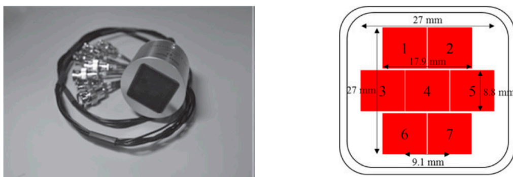
Figure 22. (a) Heavy matching layer transducer and (b) its internal configuration. Reproduced from [448] with permission from Copyright (2016) The Japan Society of Applied Physics.
