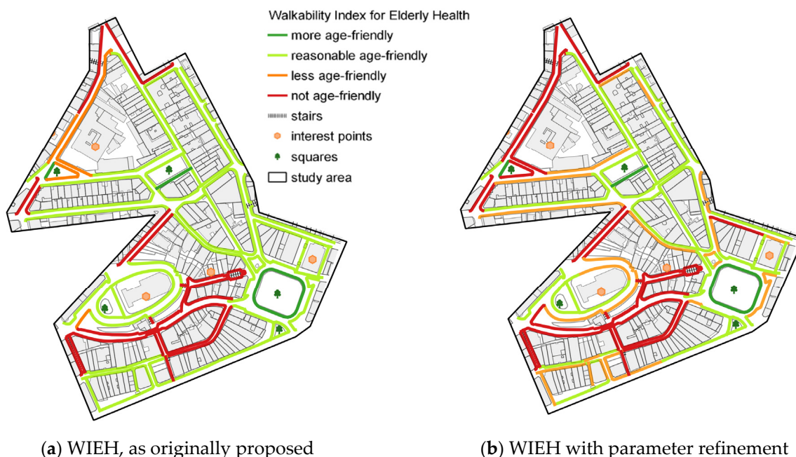
Figure 13. Comparison of WIEH ratings as per initial parameters in the previous study and the WIEH reclassifications in this study, through parameter refinement (a) WIEH as per Table 15 and Figure 9; (b) final WIEH, with the adjusted parameters, as per Table 17 (values of the ‘isw’ rating bands).
