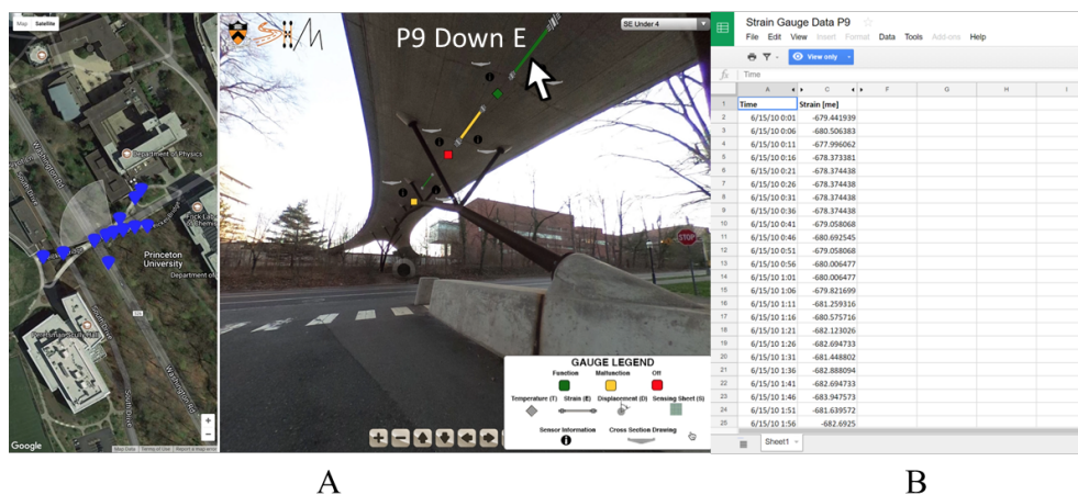
Figure 6. (A) When a user hovers over a sensor, they can see its ID as well as what it is measuring; (B) When a user clicks on the sensor they can access a database with time series.
