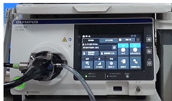
Figure 1. The new-generation endoscopy system with new technologies of texture- and color-enhancement imaging and red dichromatic imaging.
