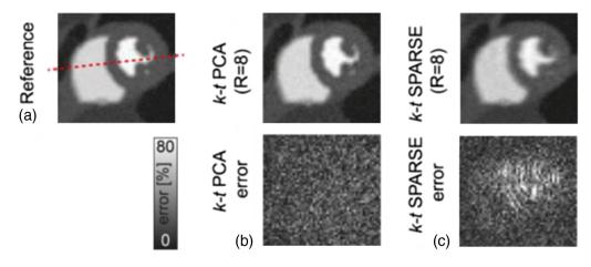
**Fig. 13** (a) Reference short-axis image of a cardiac phantom compared with (b) k-t PCA and (c) k-t SPARSE reconstruction results. In both reconstructions, the acquired imaging data were undersampled by eightfold to see the effects on reconstruction. The error distribution in k-t PCA can be seen to be more homogeneous.
