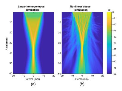
**Fig. 14** Ultrasound simulations of tissue using (a) linear and (b) nonlinear techniques showing that nonlinear techniques are valuable for understanding the distribution of acoustic energy in the body.
