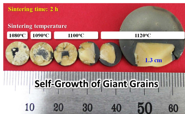
Figure 3. Variation of crystal size with sintering temperature in KNN-BCuN ceramics: The larger crystals are grown at a higher sintering temperature. The sintering time is 2 h.
