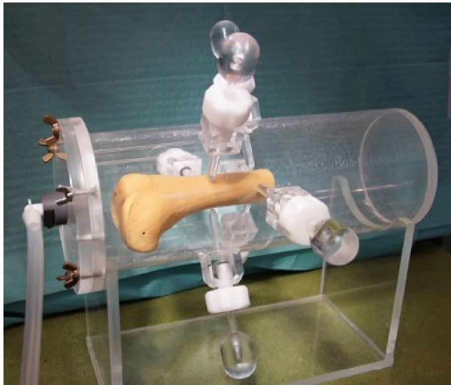
Figure 1. Picture of the custom made PMMA-cylinder with an artificial distal femur placed inside; for evacuation of air a negative pressure was applied. Afterwards the qCT was performed with the specimen inside the cylinder.
