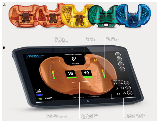
Figure 1 Pressure sensor trial inserts. (A) Variants of Verasense inserts that are available in both cruciate-retaining and posterior-stabilised designs. (B) Wireless graphical display of compartmental loads and tibiofemoral contact points in real time.
