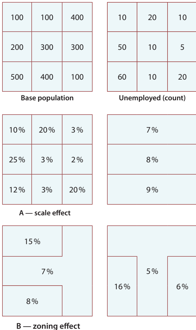
Figure 1: Illustration of the scale and zoning effect of the modifiable areal unit problem. A change in either scale or zoning changes the geographic distribution of the variable in question. In this figure, subsets A and B illustrate how different permutations of the 9 cells representing area unemployment can alter the final statistic for perceived unemployment areas.
