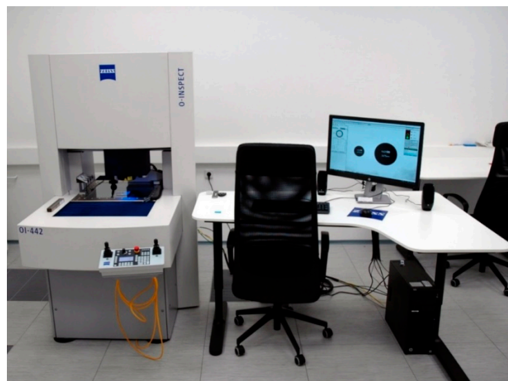
Figure 3. Zeiss O' Inspect 442 used during experiments, located at the Laboratory of Coordinate Metrology.
