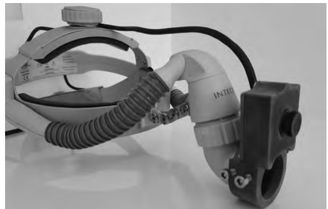
Fig. 1. 3D printed camera mounted to surgeon's headpiece.
