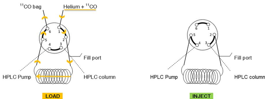
**FIGURE 1** Schematic representation of the HPLC loop applied in the  $^{11}\text{C}$ -carbonylation procedure. The yellow arrows indicate the flow direction for  $[^{11}\text{C}]\text{CO}$
