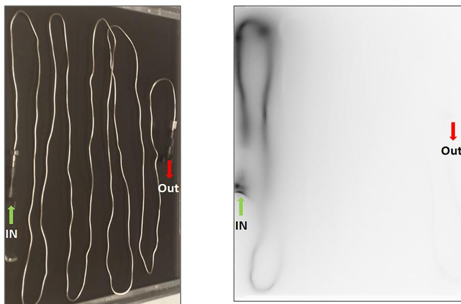
**FIGURE 2** Picture (left) and autoradiographical image (right) of the HPLC loop following entrapment of [ $^{11}\text{C}$ ]CO in the synthesis of [ $^{11}\text{C}$ ] *N*-benzylbenzamide. The arrows indicate the entry and exit points of the He carrier gas through the HPLC loop
