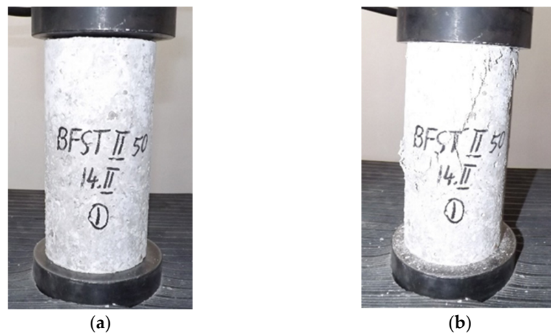
Figure 2. Concrete compressive strength testing. (a) Positioning of the test specimen; (b) compressive crack, after performing the test.
