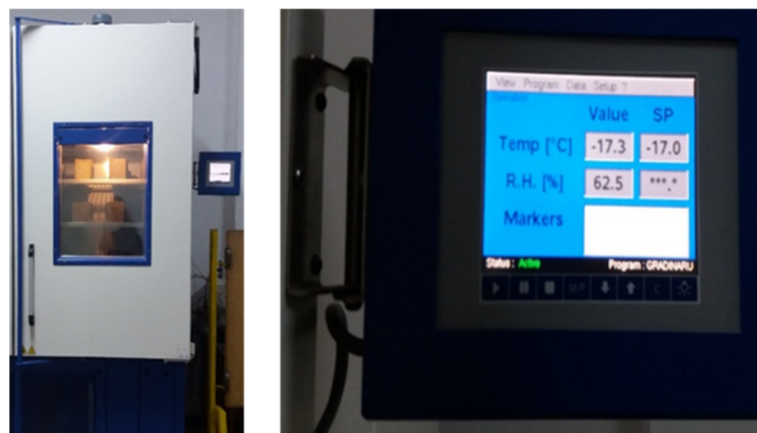
Figure 5. Refrigerated chamber used for freezing the concrete specimens.
