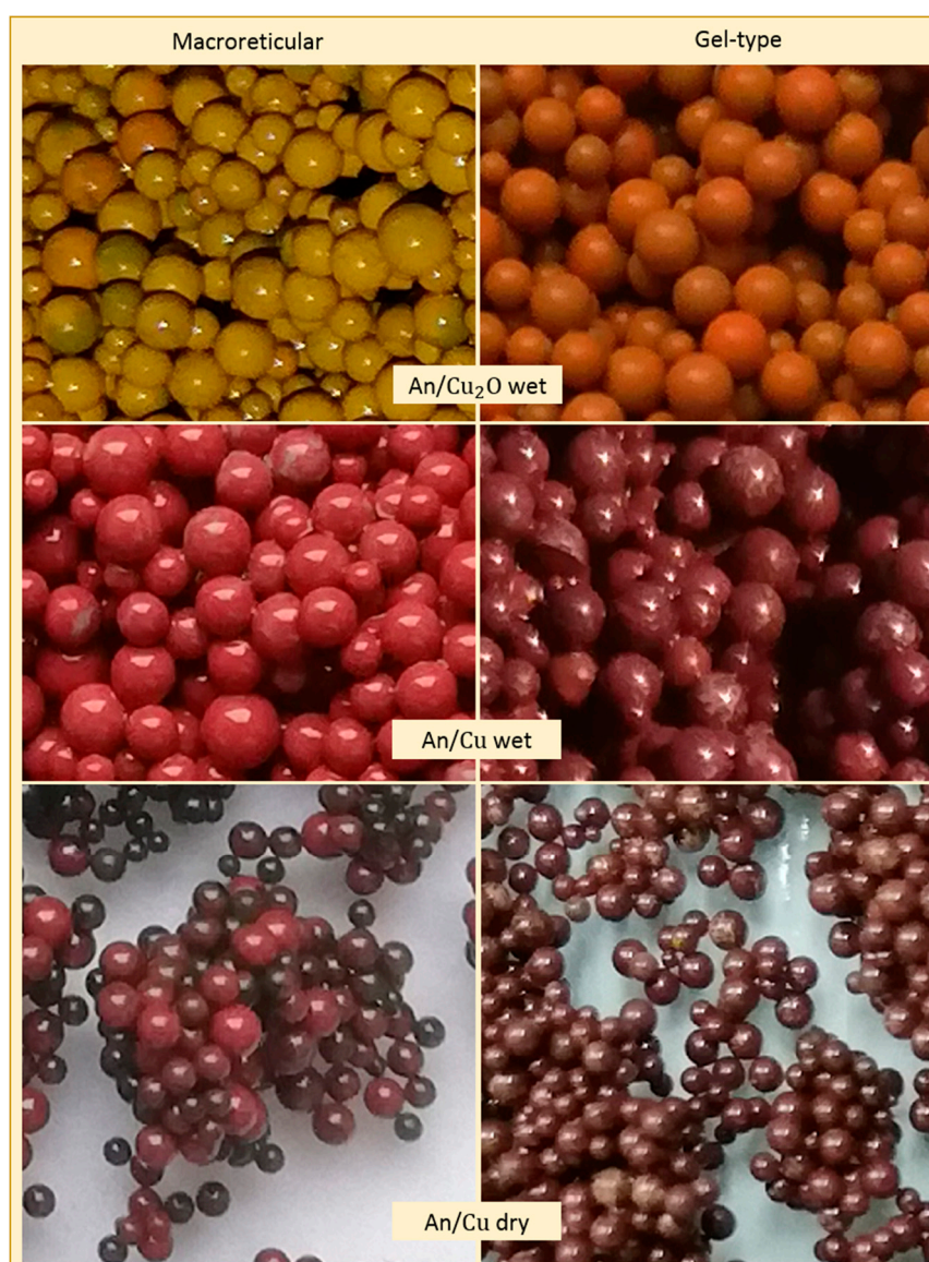
Figure 6. Photographs of examined materials: based on macroporous anion exchanger (left column) and gel-type anion exchanger (right column).
