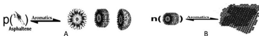
Figure 4. A) Asphaltene micellization in polar aromatic solvents. B) Asphaltene aggregation from micelles (Priyanto et al., 2001).
